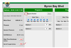
Once reaching the high moisture threshold (30%vmc), programs are disabled as indicated, and will not be re-enabled until breaching the low threshold (20%vmc).
