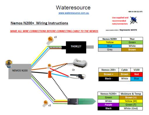
NOTE: Water meter pulse output & soil moisture sensor share BLACK ground of Nemos. Strip back 10mm, pre-twist and trim, and use orange wire nut provided.
